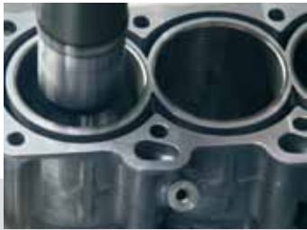
PCBN insert Cylinder boring (rough & finish)
